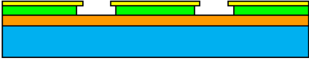
Fig. 2. Not-to-scale front view of the resist and substrate layers shown after lithography and development. The bottom layer is the silicon wafer, covered with a layer of BCB. The second layer (MMA) from the top is more sensitive than the top layer (PMMA), allowing the tunnel diode to be created by the shadow evaporation technique.
